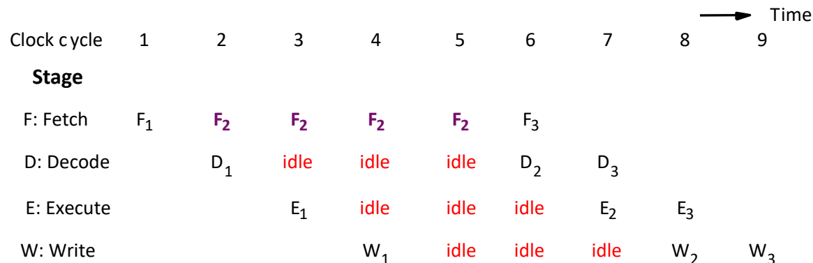
Figure: Statuses of processor stages in successive clock cycles.
